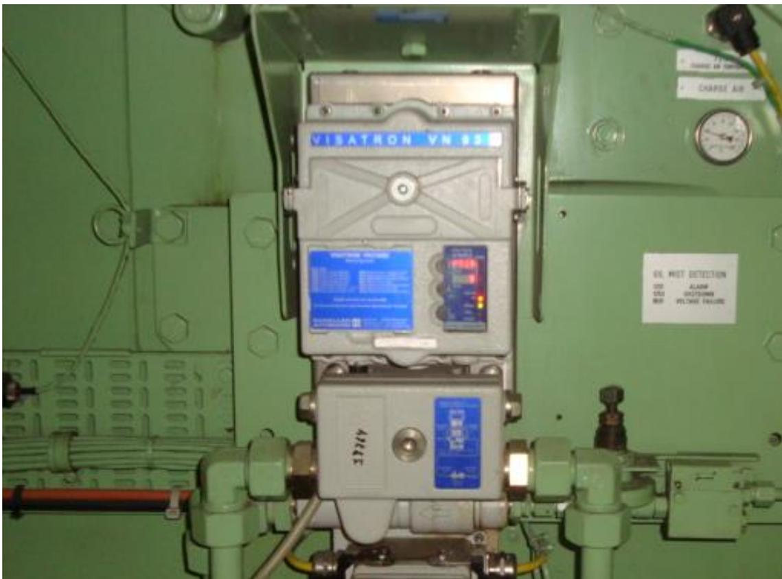
An overall mist density of the crankcase is also measured by comparing the samples with the fresh air once every rotation of the sampling valve is done. A beam of light from a common lamp is reflected through mirrors and output is measured from a photo cell.
